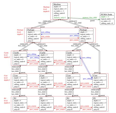
It should be noted that for PU objects, the logical index -- as computed linearly by hwloc -- is not the same as the OS index.
