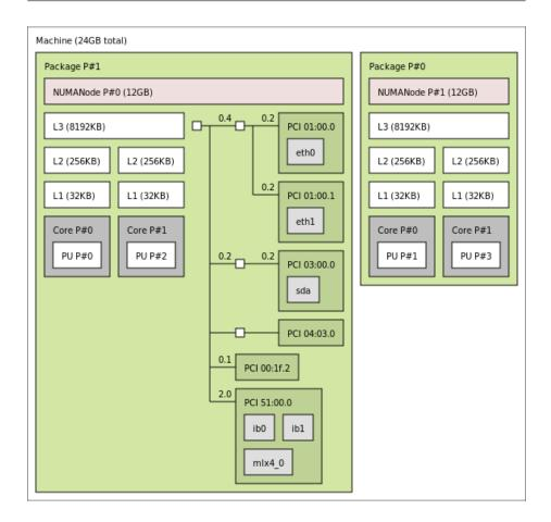
Six interesting PCI devices were discovered. However, hwloc found some corresponding software devices (*eth0*, *eth1*, *sda*, *mlx4\_0*, *ib0*, and *ib1*) for only four of these physical devices. The other ones (*PCI 102b:0532* and *PCI 8086:3a20*) are an unused IDE controller (no disk attached) and a graphic card (no corresponding software device reported to the user by the operating system).
