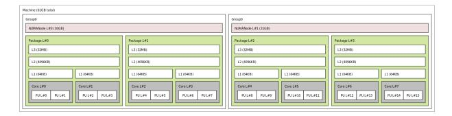
Developers using the hwloc API or XML output for portable applications should therefore be extremely careful to not make any assumptions about the structure of data that is returned. For example, per the above reported PPC topology, it is not safe to assume that PUs will always be descendants of cores.
